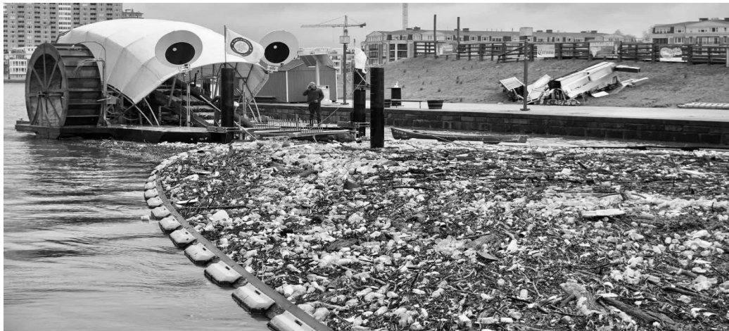
Figure 56. The mechanism for cleaning rivers from debris Mr. Trash Wheel Source: ( https://www.mrtrashwheel.com )
